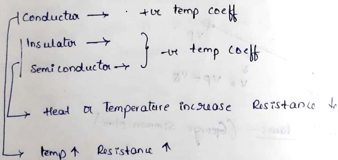
Q) calculate the Resistance of copper at  $50^\circ C$  if at  $15^\circ C$  the resistance of copper is  $0.04\Omega$  ( $\alpha_{Cu} = 0.0004/{}^\circ C$ )
