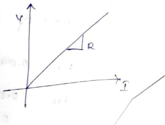
$$\Rightarrow I = \frac{V}{R} \rightarrow \frac{1}{R} = G \text{ (conductance)} \xrightarrow{\text{Unit}} \Omega$$
